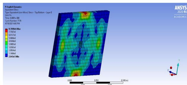
Figure 7: Bullet penetration in a unidirectional stack up
