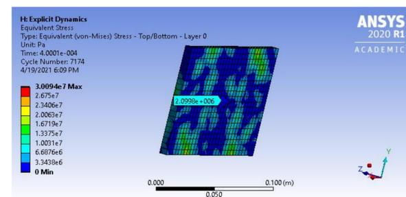
Figure 6: Bullet penetration in a 16.4-degree helical stack up
