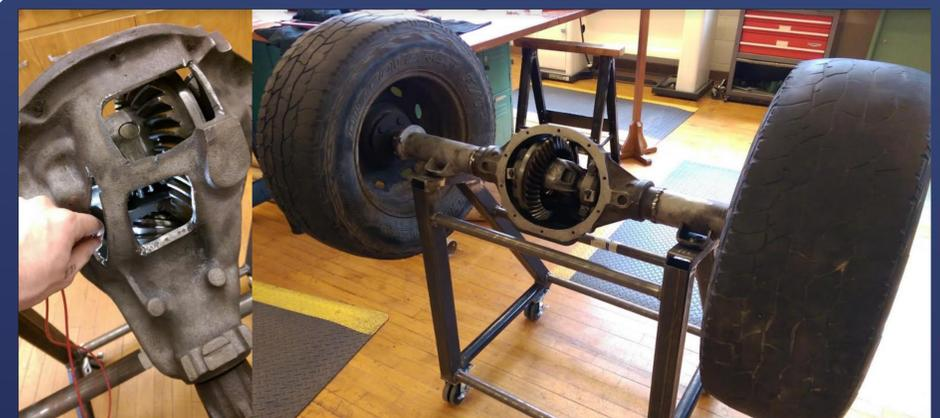
Figure 5. Custom-fabricated differential display
