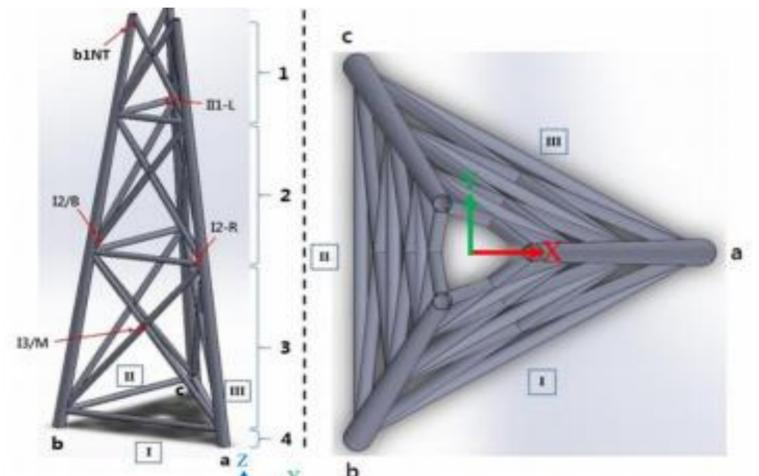
Figure 2. Three-Legged Jacket Monopile Structure
