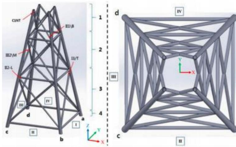
Figure 1. Four-Legged Jacket Monopile Structure Design.
