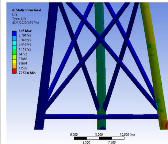
Figure 4. Four-Legged Jacket Monopile Results.
