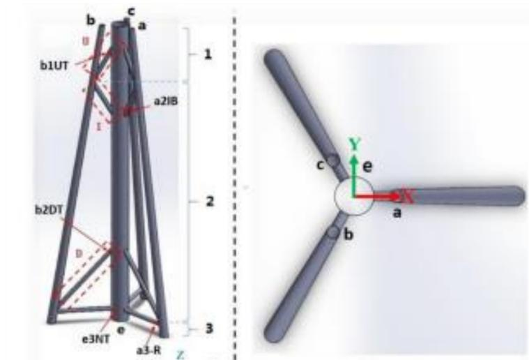
Figure 3. Three-Legged Twisted Jacket Monopile Design.
