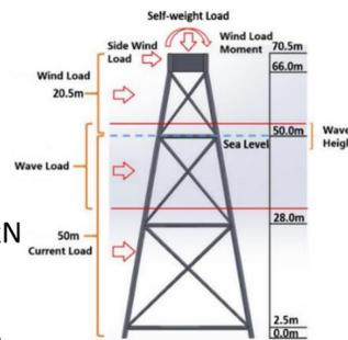
Figure 7. Structural Force Layout
