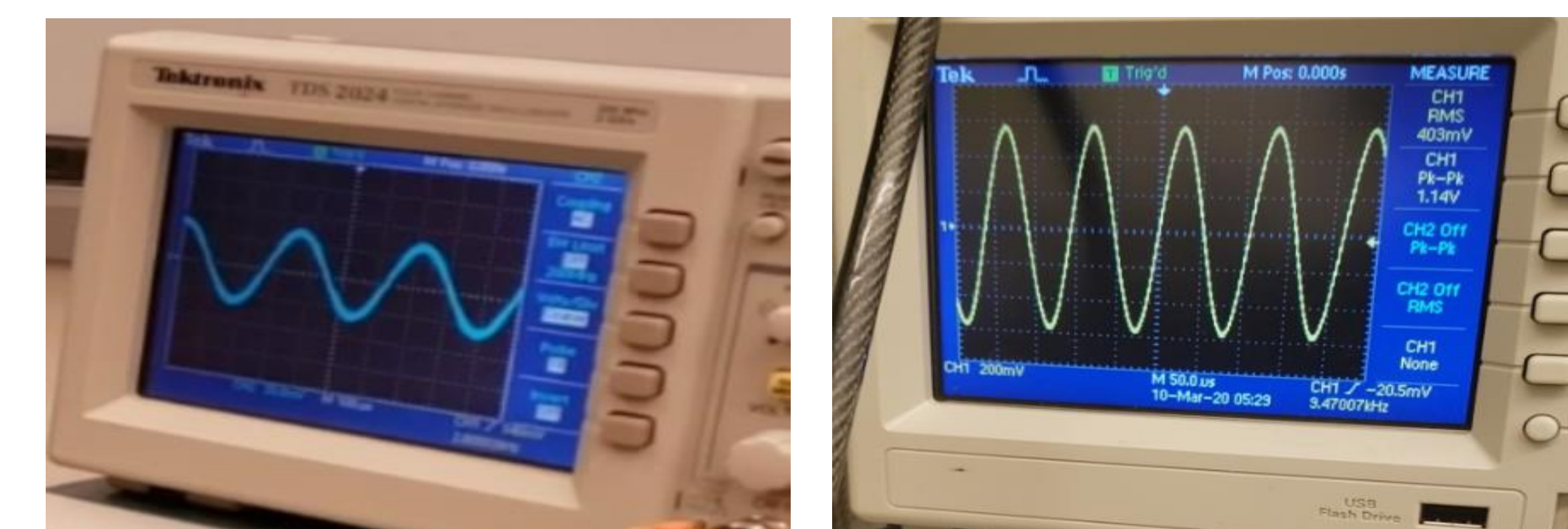
The resonant frequency at bending mode: steel (left) =4kHz Brass (right) ~10KHz
