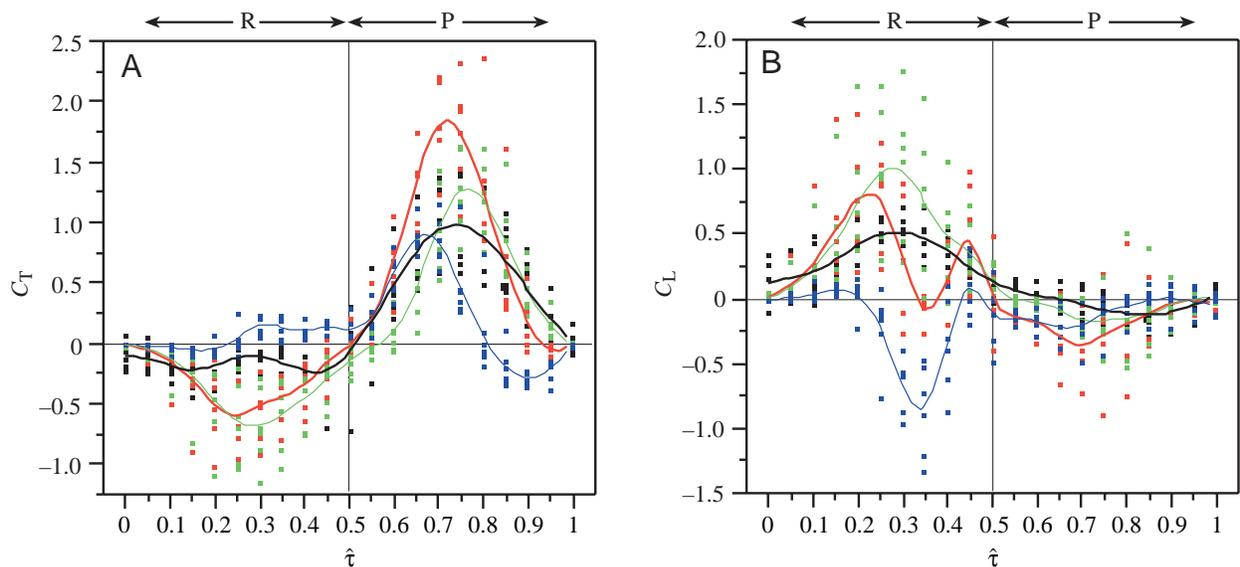
Fig. 5. Comparison of measured (black) and modeled (colored) coefficients of thrust ( $C_T$ ) and lift ( $C_L$ ) throughout a standardized stroke cycle. The time axis has been standardized within the recovery (R) and power (P) strokes. The red, green and blue lines are cubic splines of the total, circulatory and inertial forces, respectively, fit to the six different sequences (individual dots).
