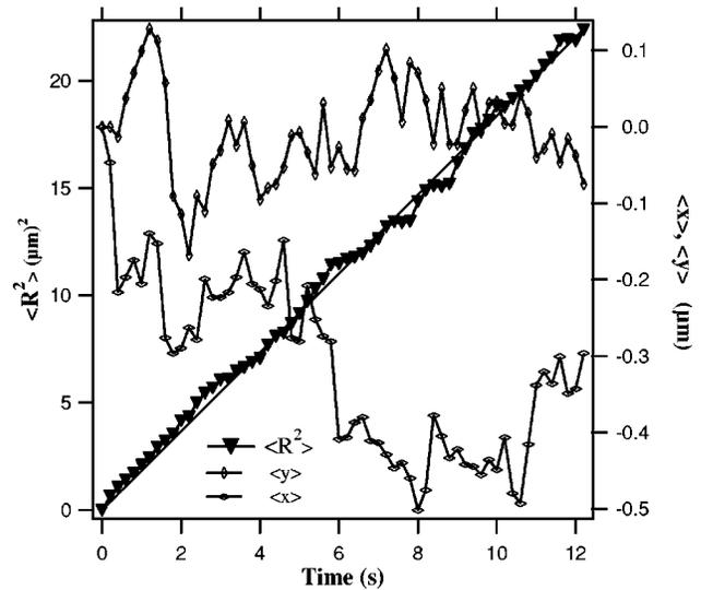
Fig. 4. Mean square displacement for 107 polystyrene spheres of diameter  $1.02 \mu\text{m}$ . Also shown are the average horizontal and vertical displacements, as well as a linear fit to the average  $R^2$  data. This fit is constrained to go through zero. The slope of this fit is  $s = 1.836 \pm 0.02 \mu\text{m}^2/\text{s}$ .
