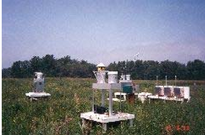
Figure 2-2. Photo of NADP sampler at the Casco Bay site (National Atmospheric Deposition Program, 2002a).
