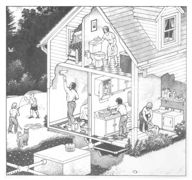
**Phosphorus treatment failure** occurs when coarse, sandy soils allow phosphorus to pass untreated through to the groundwater. In this case all the pipes and pumps are working properly, and there is no apparent evidence of malfunction. The problem lies in the inability of surrounding soils to absorb and treat the phosphorus.
