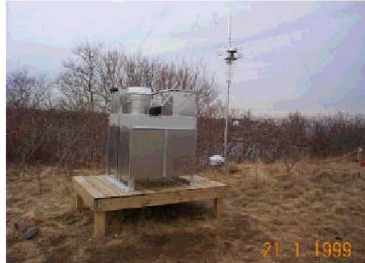
Figure 1. The UML wet/dry collector
