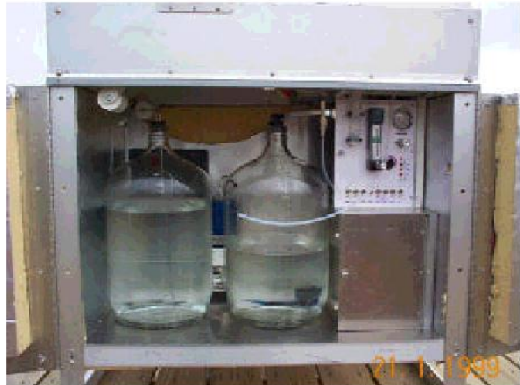
Figure 2. The interior of the dry collector
