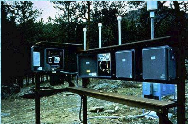
IMPROVE Modular Aerosol Sampler
