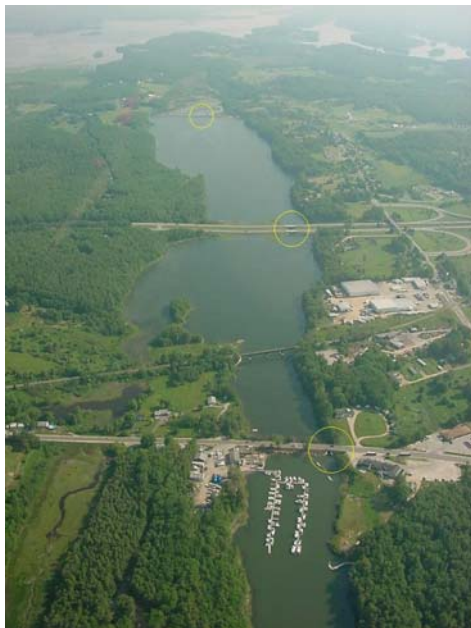
The New Meadows River Watershed Partnership is exploring the feasibility of removing causeways that restrict tidal flow and impair water quality in the river.
