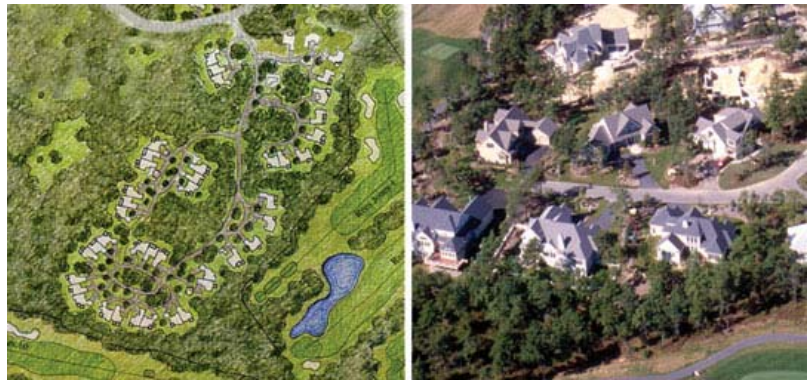
Project incorporating LID site plan principles (left – site plan, right – as built) The Pinehills, Plymouth, Massachusetts.
