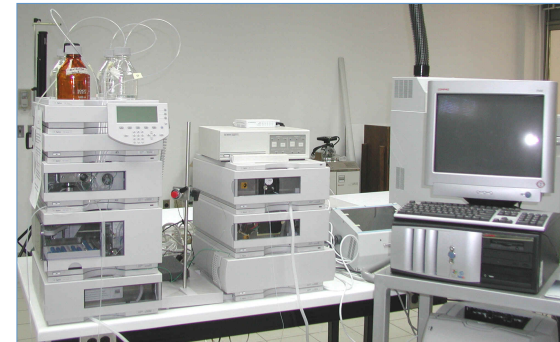
Figure 4. A high performance liquid chromatography, equipped with a diode array detector, a fluorescence detector, and an electrochemical detector (www.aub.edu.lb)
